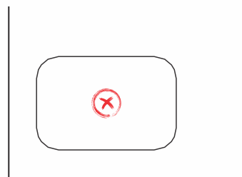
Prepare the holes on all inner corners, minimum 3mm bit diameter.
